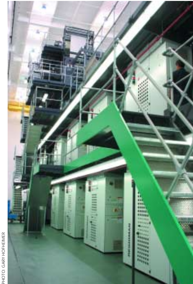
The Advertiser's new 60-foot-high printing presses can produce up to 70,000 papers per hour.
