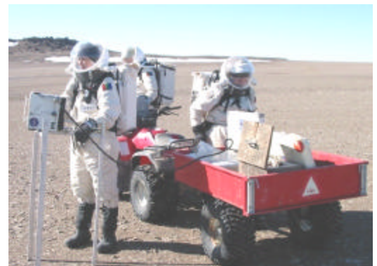
FMARS crew members take ground truth reflectance spectrometry measurements for the MISR instrument on JPL's Terra satellite.
