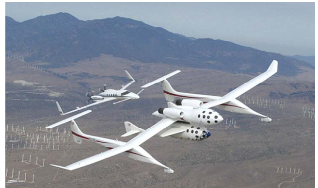
Scaled Composites White Knight launch aircraft carrying SpaceShipOne followed by a Beech Starship chase aircraft
